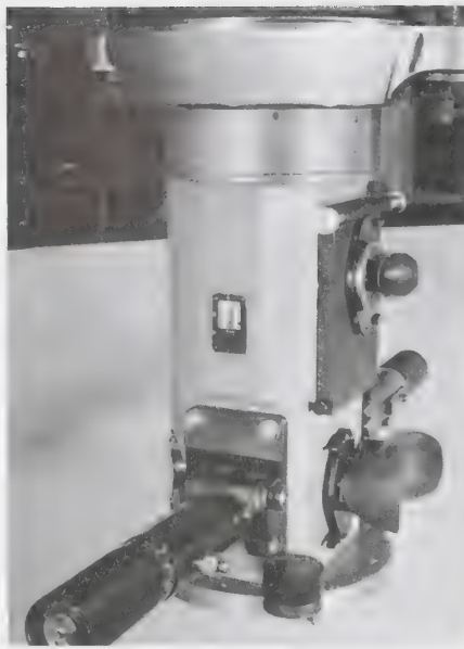
Periscope, eyepiece box and observer's station; handles control rotation about the axis, twist grips provide control of the line-of-sight elevation
